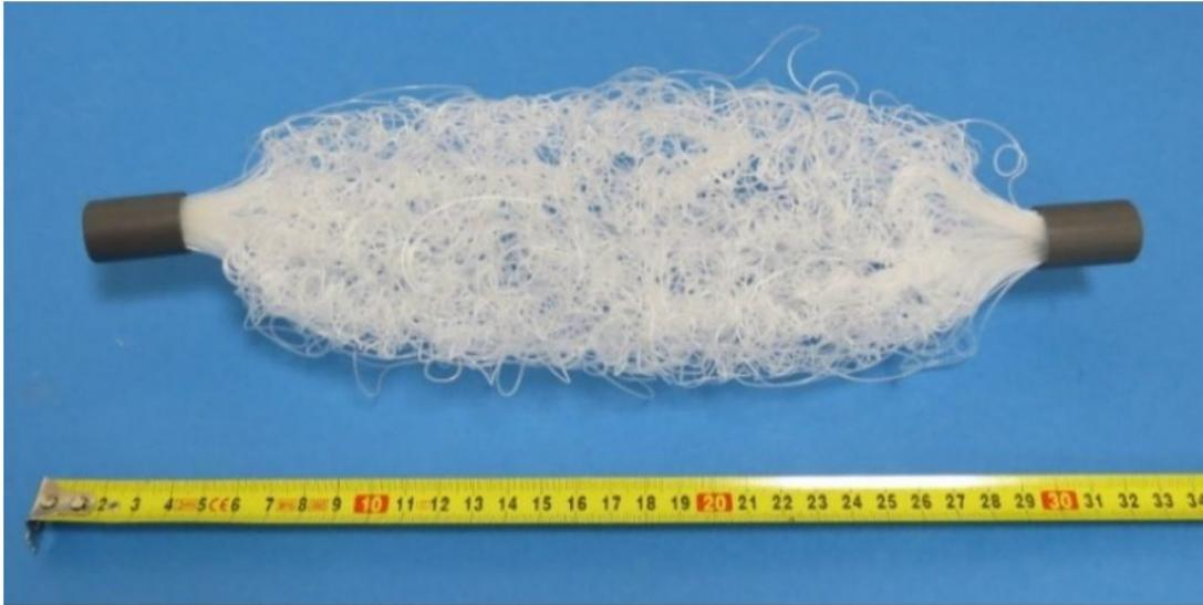
**Figure B.3:** Polymeric hollow fiber heat exchanger, condenser [5].
