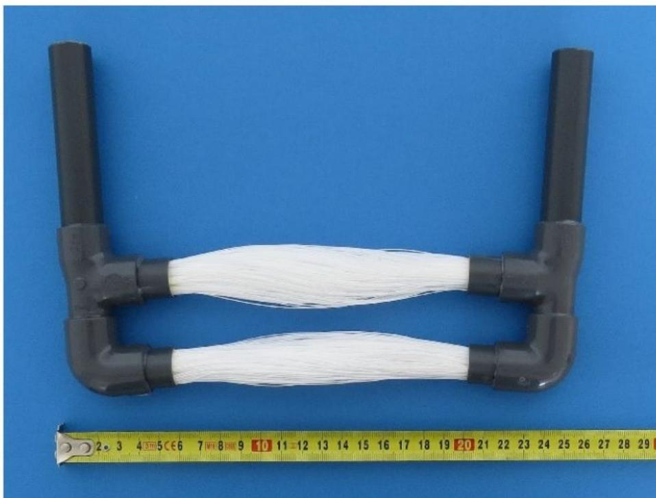
**Figure B.2:** Double-bundle membrane module MM006 [5].
