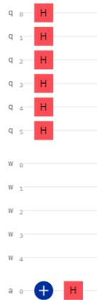
Figure 4.2: Initialisation circuit component for  $N = 64$
